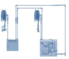
LPJET14 configuration, creating a water pressure network of cleaning point through other satellites.
