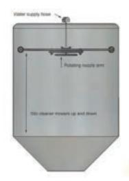
This special unit is designed for the internal cleaning and disinfection of silos or storage tanks. The unit is usually integrated into the silo.
