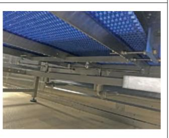
Mounting for cleaning bottom of the conveyor.
