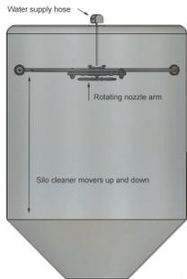
This special unit is designed for the internal cleaning and disinfection of silos or storage tanks. The unit is usually integrated into the silo. This unit is adjustable in diameter (between 2040 and 3500 mm in diameter) and has rubber wheels that run against the silo wall. The unit is connected to a hoist and a water hose that is connected to an automatic cleaning system.
