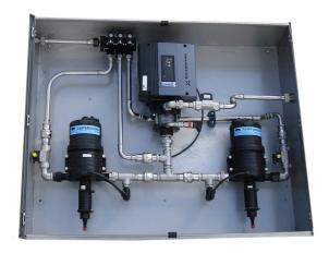
A compact design to fit directly in production areas where automatic cleaning is needed.
