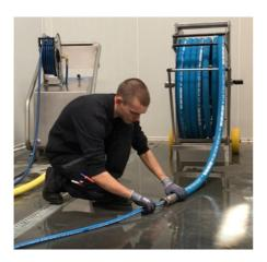
Connect the hose to the wash gun of the click & Clean tank cleaning unit.
