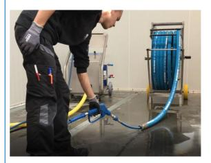
Pull the trigger of the wash-gun and automatically the nozzle pulls itself into the hose by spraying 6 rear jets and 1 front jet.
