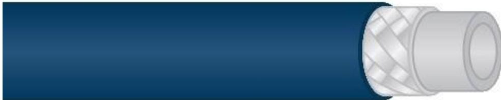
The DOSANOVA Thermoflex hose is a 5 layer, hot water wash down hose. Especially designed for the cleaning in food and dairy industry and designed for pressures up to 15 bar at 100 °C continuous use. Food grade.
